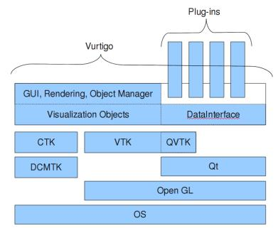
Vurtigo depends on: CTK for DICOM handling, VTK for rendering, and Qt for the GUI. The QVTK component allows the VTK render window to be placed into the Qt GUI. Both Qt and VTK make use of the OpenGL library. All of Vurtigo's plugins have one class derived from the DataInterface class.
